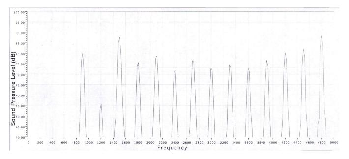
As shown above, the fundamental frequency is 975 Hz, and there are more than 4 harmonic peaks between 1 and 4 kHz. All harmonic peaks are within  $\pm$  15 dB of the fundamental frequency
