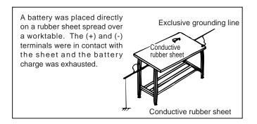
When batteries are to be used near protective materials, take every possible care to ensure that the (+) and (-) terminals of the batteries or PC boards, etc. on which batteries are mounted do not touch these protective materials directly.
