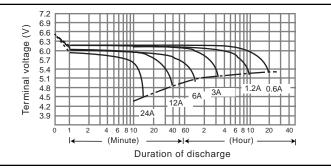
Duration of discharge vs. Discharge current (Note)
