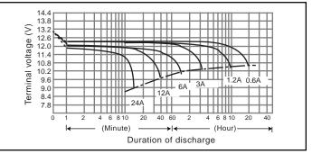
Duration of discharge vs. Discharge current (Note)
