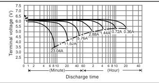
Duration of discharge vs. Discharge current (Note)
