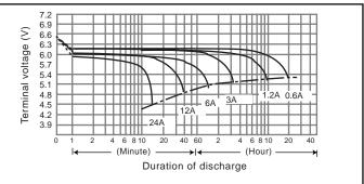
Duration of discharge vs. Discharge current (Note)
