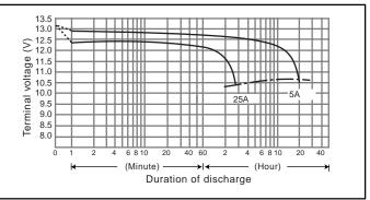
Duration of discharge vs. Discharge current (Note)
